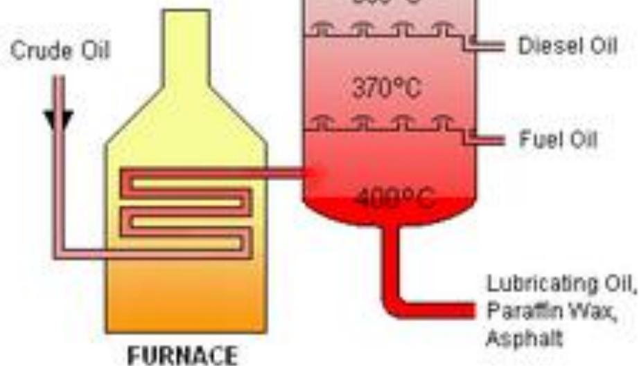
To separate a mixture of liquids with closer boiling points or those containing several components
