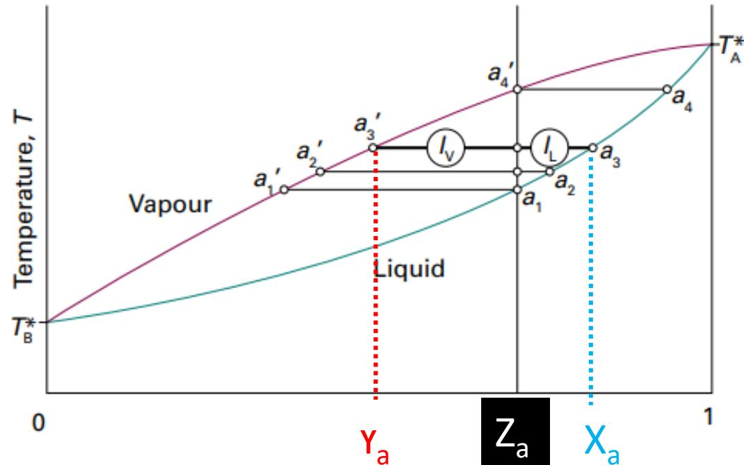
These isopleths show the change in liquid and vapor content at different temperatures for a given  $Z_a$
