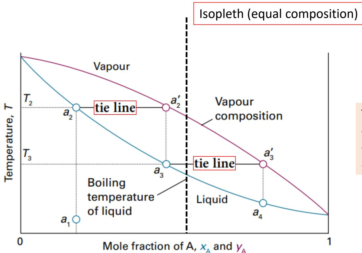
The red line is the composition of the vapor in equilibrium with the liquid at each temperature
