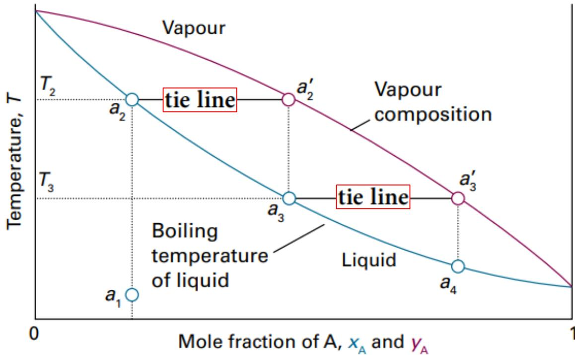
The red line is the composition of the vapor in equilibrium with the liquid at each temperature
