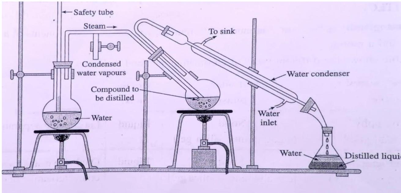
Steam distillation is used to distill temperature-sensitive, water-insoluble compounds.
