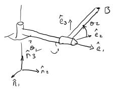
3.10: A compound solar panel on a satellite is shown. The inner panel undergoes a rotation about the vertical axis, e2, while the outer panel undergoes a rotation about the e1 axis.
