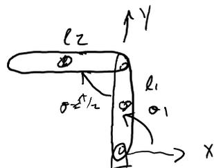
Robot link w/  $\theta$  fixed, find velocity when  $\theta_1 = 180^\circ$  (starts @ rest)
