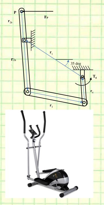
$T_4 = -100$ Ncm resistance torque,  $\theta_4$ \_dot = +20rpm,  $\theta_{2b}$ \_dot = +10rpm, r<sub>1</sub> = 1150, r<sub>2a</sub> =850, r<sub>2b</sub> =450,  $\theta_{2b}$  = 100 deg, r<sub>3</sub> = 950, r<sub>4</sub> = 400
