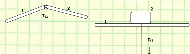
For bodies not connected immediately by a joint, the technique relies on Kennedy's Theorem:
