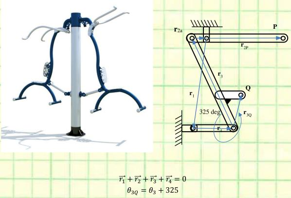
$\begin{array}{l} r_1 = 510 \text{ cm}; r_2 = 120 \text{ cm}; r_3 = 538 \text{ cm}; r_4 = 300 \text{ cm}, r_{2P} = 500 \text{ cm}; r_{3Q} = 150 \text{ cm}; \\ \theta_1 = 250 \text{ deg}; \theta_2 = 0 \text{ deg}; \theta_3 = 117 \text{ deg}; \theta_4 = 0 \text{ deg}; \text{ branch} = -1 \\ \theta_{2\_dot} = 1 \text{ rad/s} \end{array}$
