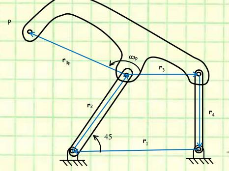
Given  $r_1 = 161$  cm;  $r_2 = 141$  cm,  $r_3 = 120$  cm,  $r_4 = 100$  cm,  $\theta_2 = 45$ deg,  $\dot{\theta}_2 = .5$  rad/s,  $r_{3p} = 200$ ,  $\alpha_{3p} = 135$ deg, find the input torque required at link 2 to lift a 1000 kg. load placed at point P.
