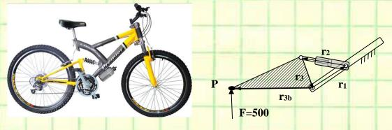
$\begin{aligned} \mathbf{r}_1 &= 20 \text{cm}, \, \mathbf{r}_2 = 25 \text{ cm}, \, \mathbf{r}_3 = 35 \text{ cm}, \\ \theta_1 &= 50 \text{ deg}, \, \theta_2 = 128.5 \text{ deg}, \, \theta_3 = -85.6 \text{ deg}, \, \theta_{3b} = 175 \text{ deg}, \\ \mathbf{r}_2 \text{ dot} &= 75 \text{cm/s}, \, \mathbf{V}_{\text{px}} = 5 \text{ cm/s}, \, \mathbf{V}_{\text{py}} = 125 \text{ cm/s}, \end{aligned}$
