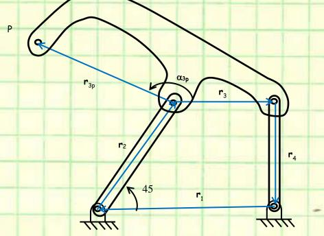
Given  $r_1 = 161$  cm;  $r_2 = 141$  cm,  $r_3 = 120$  cm,  $r_4 = 100$  cm,  $\theta_2 = 45$ deg,  $\dot{\theta}_2 = .5$  rad/s,  $r_{3p} = 200$ ,  $\alpha_{3p} = 135$ deg
