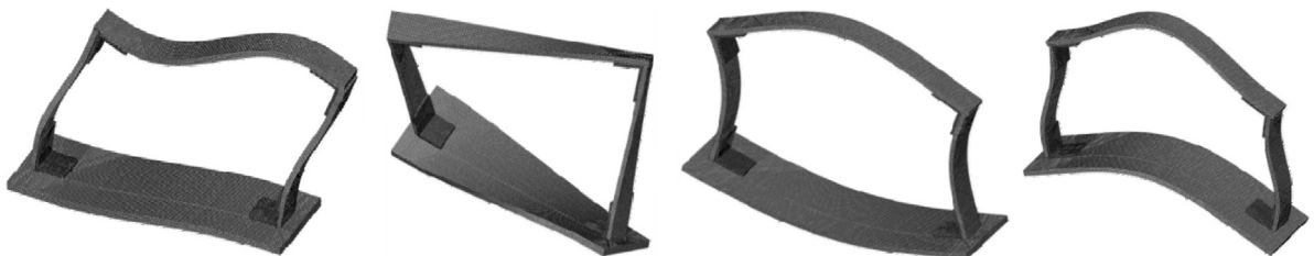
Fig. 10. First four resonant mode shapes predicted by the tied node FE model.
