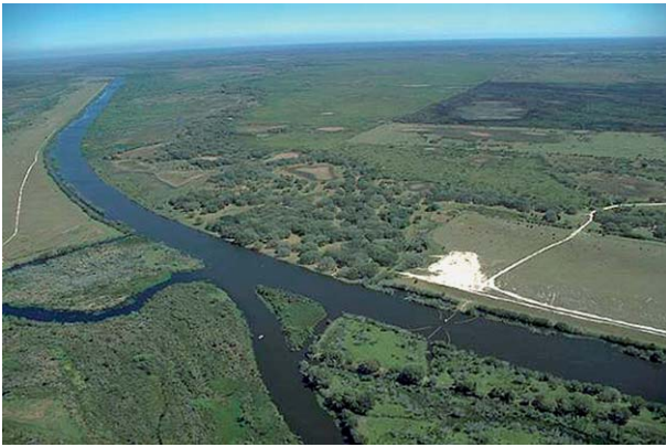
Figure 3 Aerial view of the channelized Kissimmee River, FL, USA. Photo courtesy of Pat Lynch, SFWMD.
